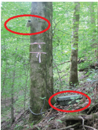
Figure 4. Acoustic sampling device and data recorder used to record pulses emitted by bats at one of the study sites.
