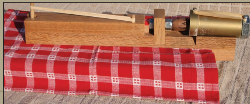
Figure 7. Texas Inertia Cracker. Dowel rod attached to red plunger at left is pulled back which further stretches the rubber band and is then released. This shatters the nut shell without appreciable damage to the kernel.
