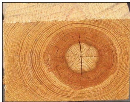
Figure 1. This cross-section of a southern pine crosscut clearly shows the annual growth rings. The heartwood, shown in the center of this piece, is a slightly darker pumpkin color than the sapwood.
